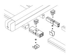
Easy clip intermediate joints (for 2 & 3 module systems)
